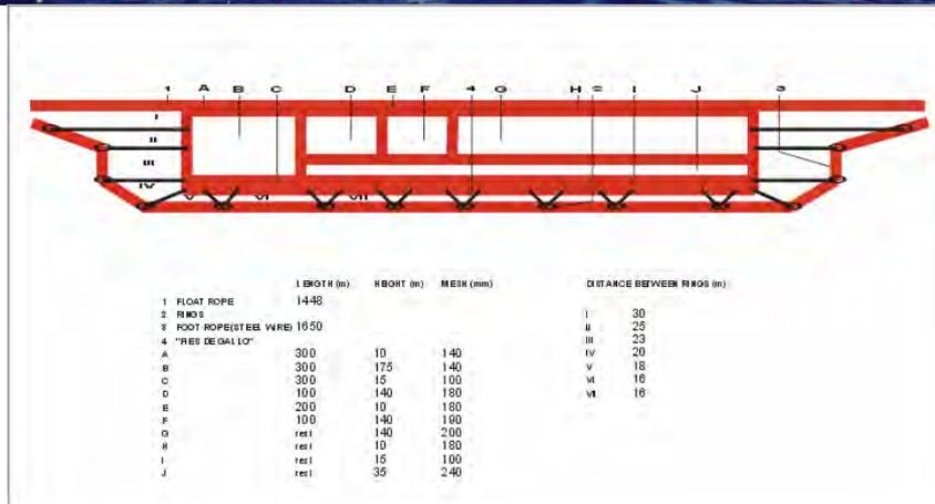
**Figure 11.-** Spanish vessel of purse seine fishing of bluefin tuna and Scheme.
