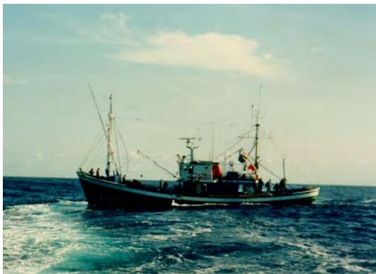
**Figure 6. Spanish vessel Baitboat for tuna fishing**
